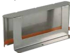
Rinnai stainless steel flue diverters are an accessory that can be fitted to an external Rinnai INFINITY water heater to expel combustion gases in either a sideways or upwards direction. The flue diverter is fitted with screws to the flue terminal of the water heater<sup>1</sup>.
