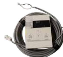
Extension cabling is available as an accessory from Rinnai. Alternatively, a two core sheathed (double insulated) flex with a minimum cross sectional area of 0.5 mm<sup>2</sup> may be used.
